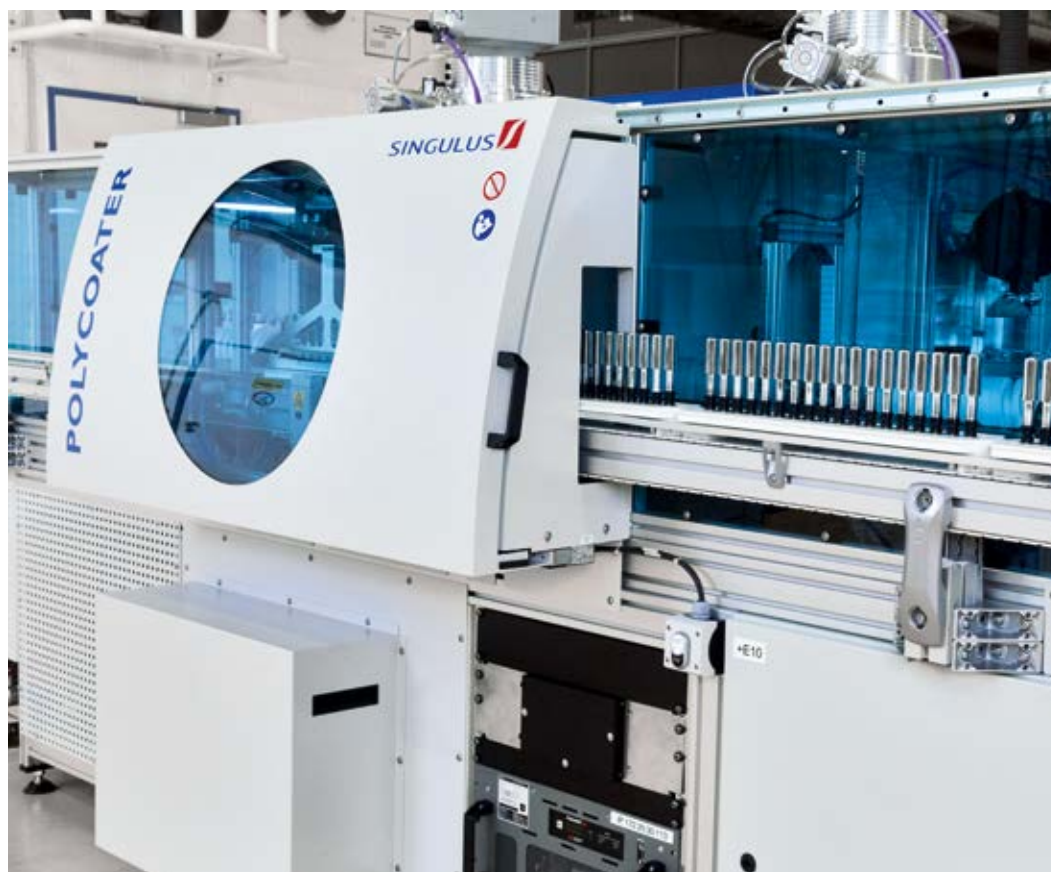
POLYCOATER Inline vacuum coating system for the sustainable production of consumer goods for cosmetics and automotive.
