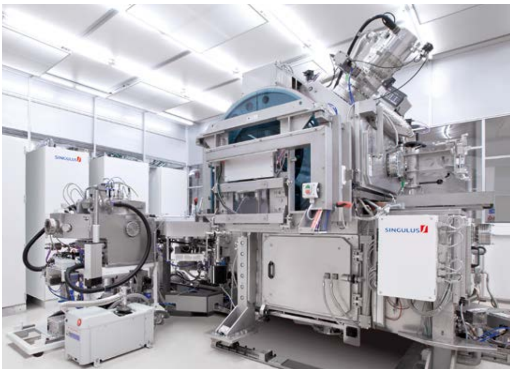
TIMARIS Ultra-high vacuum deposition system for the semiconductor industry.
