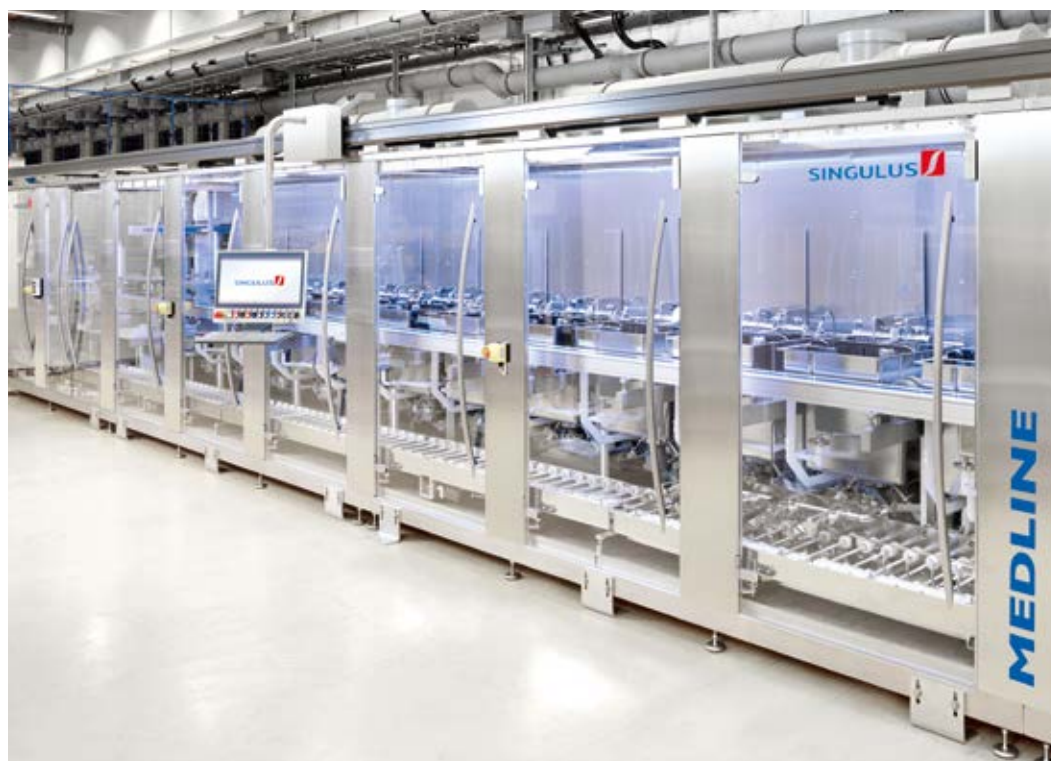
MEDLINE Cleaning and coating system for medical parts e.g. daily lenses or pacemakers.
